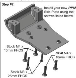
Once the Skid Plate is bolted in place, reinstall the front bumper / bumper support braces using stock screws and lock nuts.
