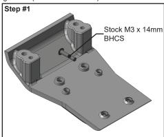
Reinstall the stock M4 x 14mm BHCS into the stock #25910 arm mount cover before bolting your new *RPM* Skid Plate in place.
