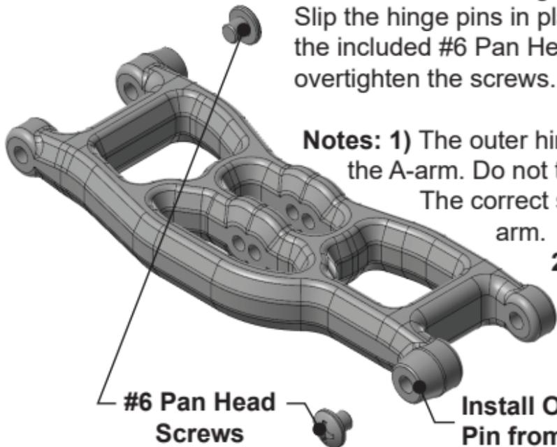
**Notes:** 1) The outer hinge pin will only go in from one side of the A-arm. Do not try to force it in from the wrong side. The correct side is from the conical side of the arm.
