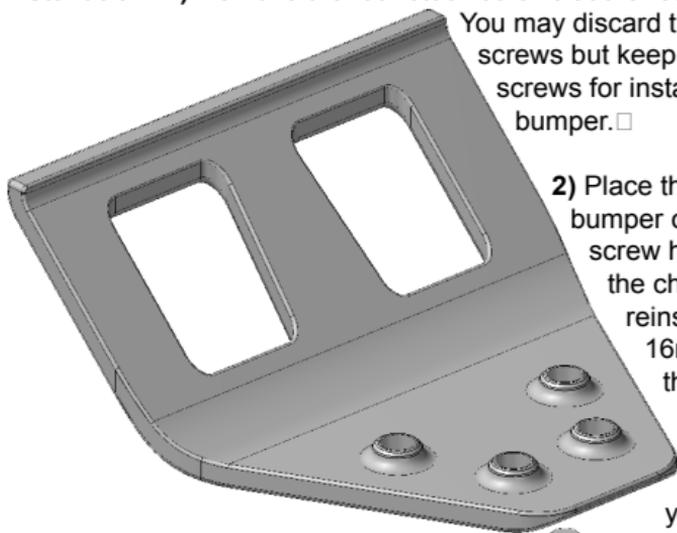
2) Place the **RPM** Rear bumper over those 4 screw hole locations in the chassis and reinstall the two M3 x 16mm screws in their original locations. Replace the M3 x 10mm screws you removed earlier with the two M3 x 12mm screws included in this kit.
