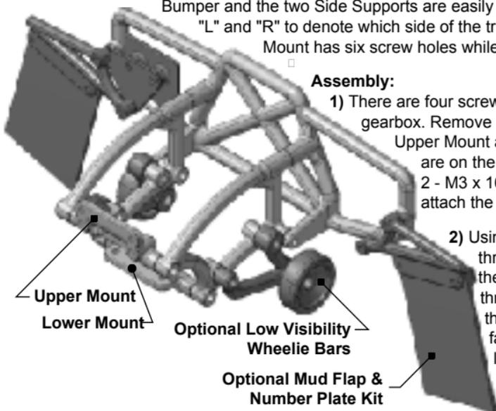
1) There are four screws that attach your stock rear shock tower to the gearbox. Remove and discard these 4 screws. Identify the **RPM** Upper Mount and rotate it so the Side Support mounting ears are on the bottom and the flat towards the shock tower. Use 2 - M3 x 16mm (top) and 2 - M3 x 25mm screws (bottom) to attach the Upper Mount to the shock tower.
