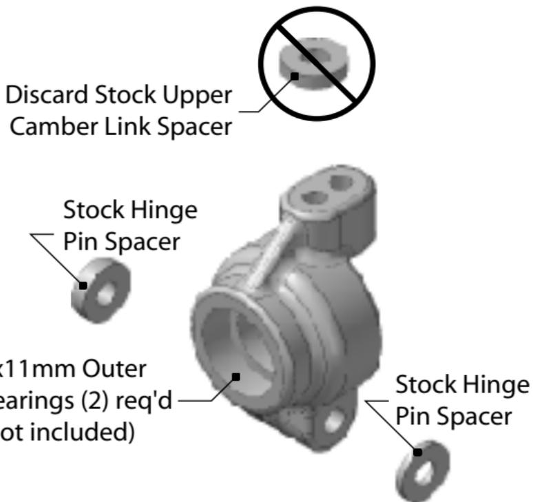
Notes: Discard stock 10mm Outer Bearings and replace with 5x11x4mm bearings (not included). Stock 15mm Inner Bearings (not included) must be reused. Install clean (or new) bearings only.
