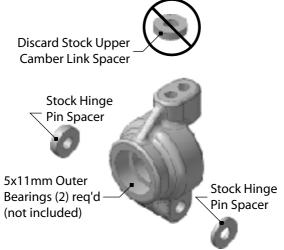
Notes: Discard stock 10mm Outer Bearings and replace with 5x11x4mm bearings (not included). Stock 15mm Inner Bearings (not included) must be reused. Install clean (or new) bearings only.
