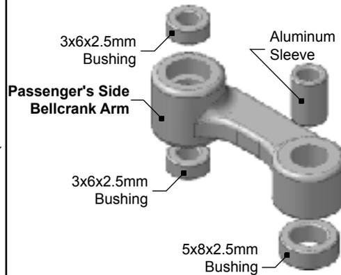
Trim any extra plastic off of the bellcrank arm, then trim bushings from sprue flush for accurate fit. Press all shown bushings into their respective locations.
