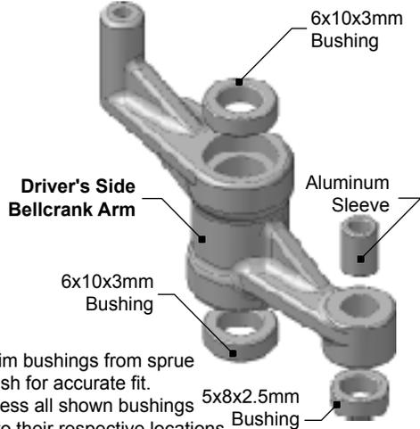
Trim bushings from sprue flush for accurate fit.
