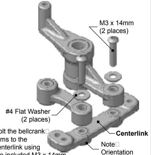
Bolt the bellcrank arms to the centerlink using the included M3 x 14mm screws and #4 washers (smooth side towards centerlink). Note the orientation of both bellcranks as well as the centerlink. The large centerlink bosses should face down. Caution: Do not over-tighten the screws. The assembly should move freely.
