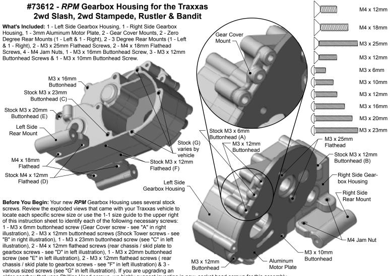
older gearbox that uses Phillips Head screws, we highly suggest investing in new, socket head screws for this assembly.
