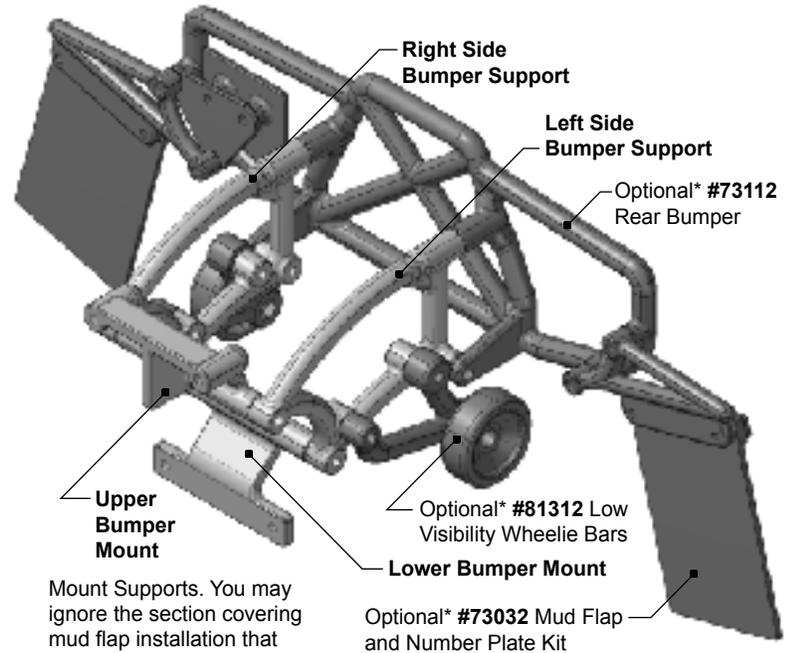
Mount Supports. You may ignore the section covering mud flap installation that came with your Wheelie Bars. For reference, an optional\* **RPM** Mud Flap and Number Plate Kit is available for the SCTE (**RPM #73032**). However, they mount to the optional\* **RPM** SCTE Rear Bumper (**RPM #73112**) as shown in the illustration above.
