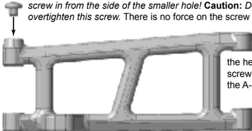
cause it to come out. Tighten until the head of the screw just touches the A-arm, then stop.
